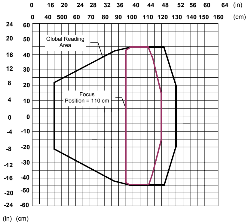
DS6400-105-0XX (Oscillating Mirror) – Resolution: 0.30 mm/12 mils
